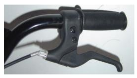
2. Insert the brake cable wire into the slot in the front of the brake lever and then remove your hand. The brake cable cap will automatically spring back into the slot on the front of the brake lever assemble.
