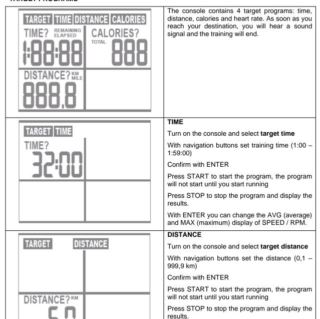
With ENTER you can change the AVG (average) and MAX (maximum) display of SPEED / RPM.
