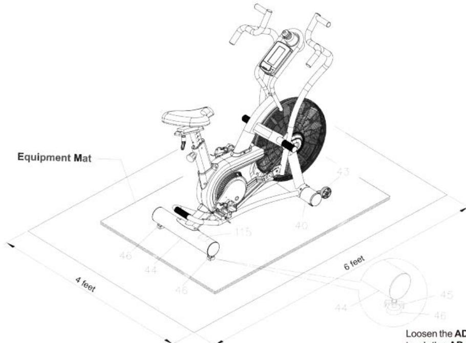
Loosen the **ADJUSTMENT LOCKS(45)** until they touch the **ADJUSTABLE FOOT(46)**. Adjust the **ADJUSTABLE FOOT(46)** for leveling. Tighten the **ADJUSTMENT LOCKS(45)** securely against the **REAR STABILIZER(44)** to lock the **STANDS (51)** in position.
