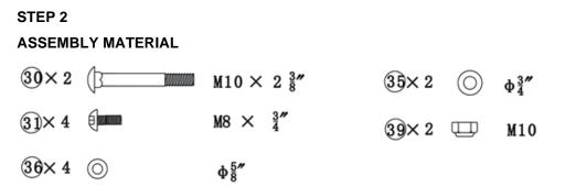
Attach the frame (3) and the frame (9) to the frame (4) and connect them 2x bolts (30), 2x washers (35) and 2x nuts (39).
