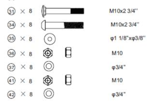
Connect the columns (1) using the connection frame (2) and 8x bolts (31), 2x plates (9), 8x washers (42) and 8x nuts (41).
