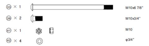
Attach the leg curl frame (7) to the seat frame (4) using the axis (28), 2x bolts (38) and 2x washers (42).
