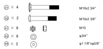
Connect the seat frame (4) to the front pillar (5) using 2x bolts (32), 2x washers (44), 2x washers (42) and 2x nuts (41).
