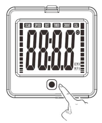
Press the MODE button to change the displayed data: SPEED, DISTANCE, TIMER, COUNT, CALORIES.
