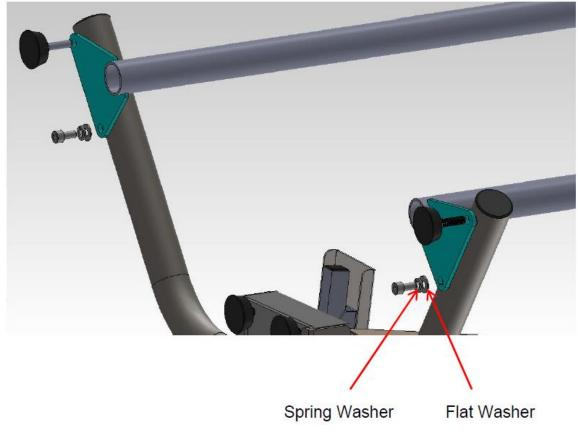
Use a 6 mm Allen key and M8x20L bolts and washers to connect the handles. Do not tighten yet.
