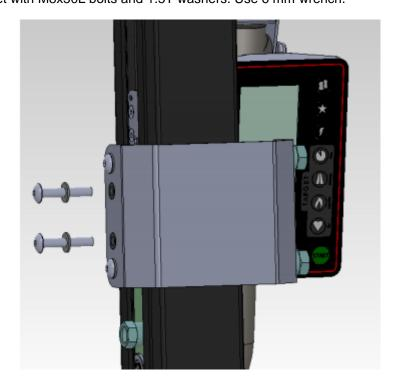
**Step 4**Attach the second bracket, align the holes as shown.
