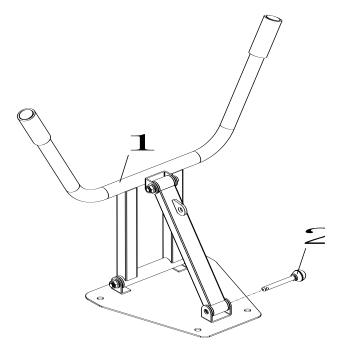
Secure the handlebar (1) with bolt (2).
