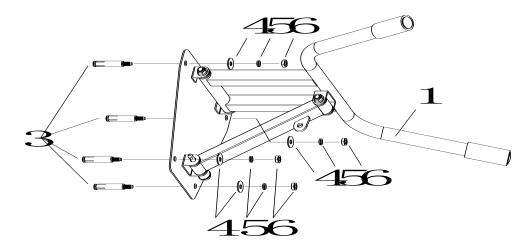
Drill the appropriate holes in the wall. Attach the wall bars with the screws (3), washers (4 and 5) and nuts (6).
