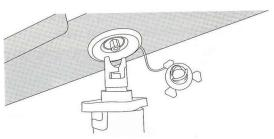
6. Connect the air tube to the valve.
