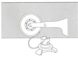
5. Press the valve and turn is counterclockwise by 45 degree.
