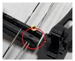
Then attach the limbs to the crossbow stock and secure with 2x Allen screws.
