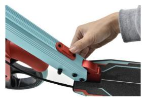
Use an Allen key to adjust the folding mechanism so that it is properly tightened.
