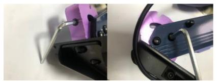
Attach the handles. The handles are secured with pins.
