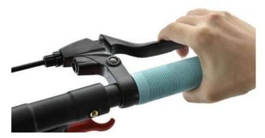
You can adjust the sensitivity of the brake using the thread on the underside.
