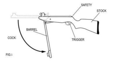
**Warning**: Hold the barrel firmly during cocking so that it does not suddenly spring back and cause injury. Be careful when breaking and keep your fingers away from moving parts of the mechanism. (Fig. 2)
