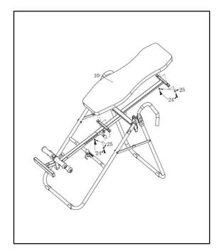
Attach the Backrest Pad (10) to the Backrest Support Frame (3) with 4x Washers M8 (24) and 4x Hexagonal Bolts M8x35 (24).
